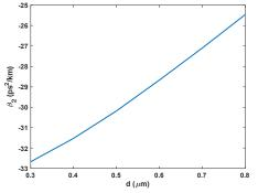
Figure (4): The relation between  $\beta_2$  and the hole diameter, d.
