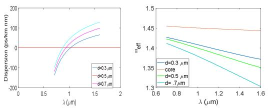
Figure (2): The dispersion curve and n<sub>eff</sub> for different values of hole diameter.
