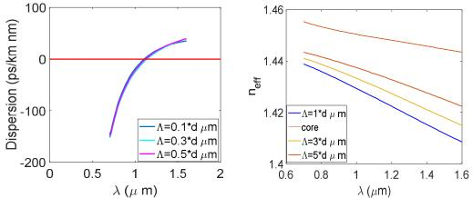
Figure (1): The dispersion curves (left), and  $n_{eff}$  (right), changes with wavelength at d=0.3 um, N=5.
