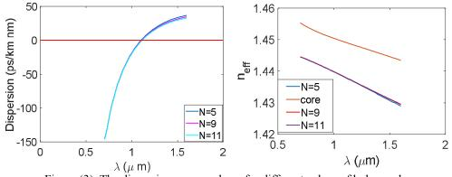
Figure (3): The dispersion curve and  $n_{reff}$  for different values of hole number.
