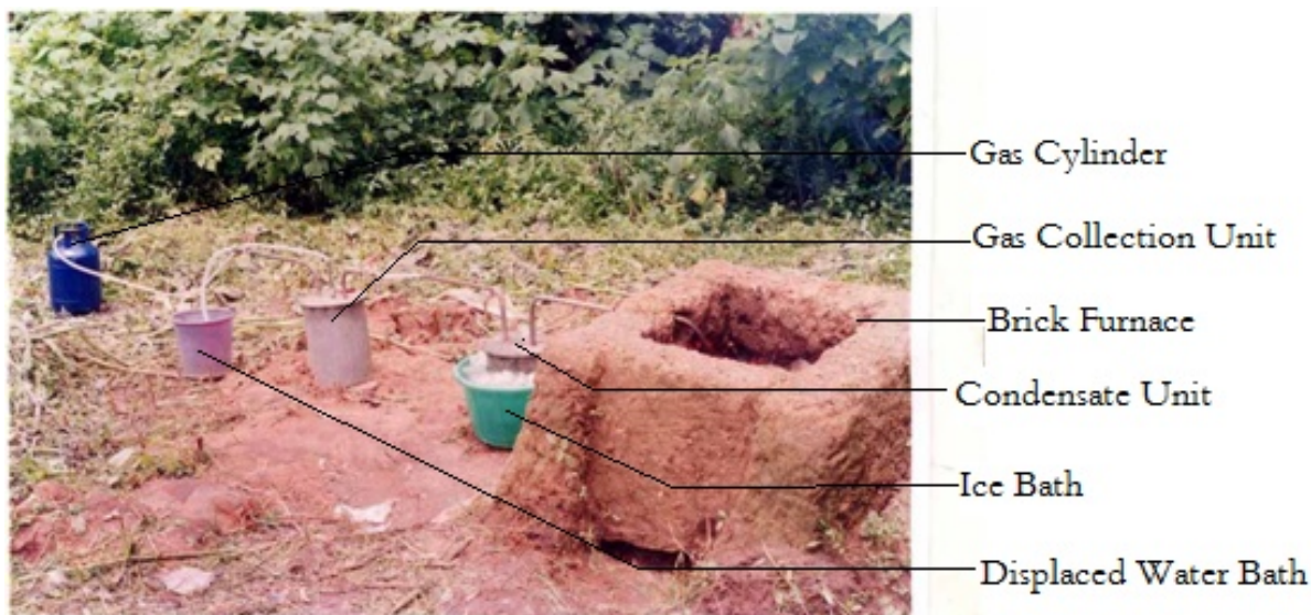
Plate 1. Pyrolysis chain assembly
