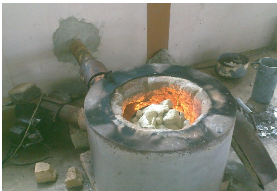
Plate 1: Heating of the Limestone Samples in a Furnace
