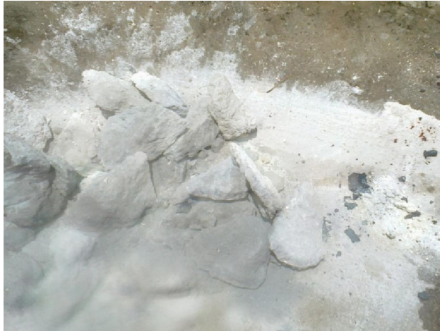
Plate 2: Hydration of the Obajana Limestone Samples with water
