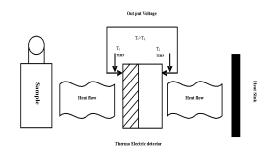
Fig. 1 Principle of measuring the heat by Microcalorimeter.
