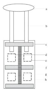
**Fig.3** Cross sections of the double twin microcalorimeter; (a) Ampoule lifter ; (b) Tubes through which the calorimeters are charged; (c) Steel can; (d) Top reference ampoule position; (e) Top measuring ampoule position; (f) Heat flow breaker. (g) Bottom reference ampoule position; (h) Bottom measuring ampoule position.
