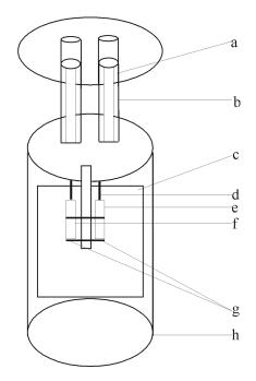
**Fig.2** One unit of TAM III multi-channel isothermal micro calorimeter ; (a) Ampoule Lifter; (b) Equilibration Tube; (c) Heat Sink; (d) Ampoule lifter; (e) Sample measuring cup;(f) Reference measuring cup; (g) Thermoelectric modules; (h) Cylinder.
