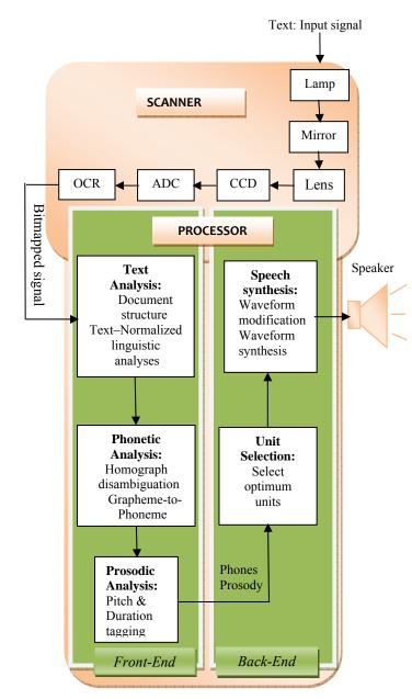
Figure 9. Block diagram of reading machine
