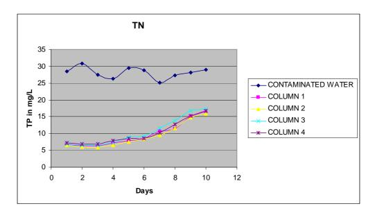
Fig. 5. Quantity of removed TN (mg/L)
