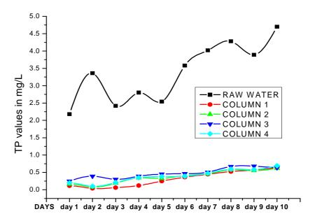
Fig.4. Quantity of TP removed (mg/L)
