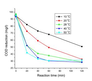
Figure4: Effect of temperature on the COD reduction
