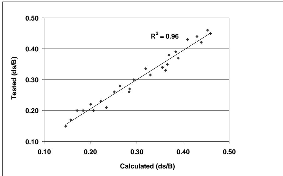
Figure 10. Comparison of calculated and tested scour depth
