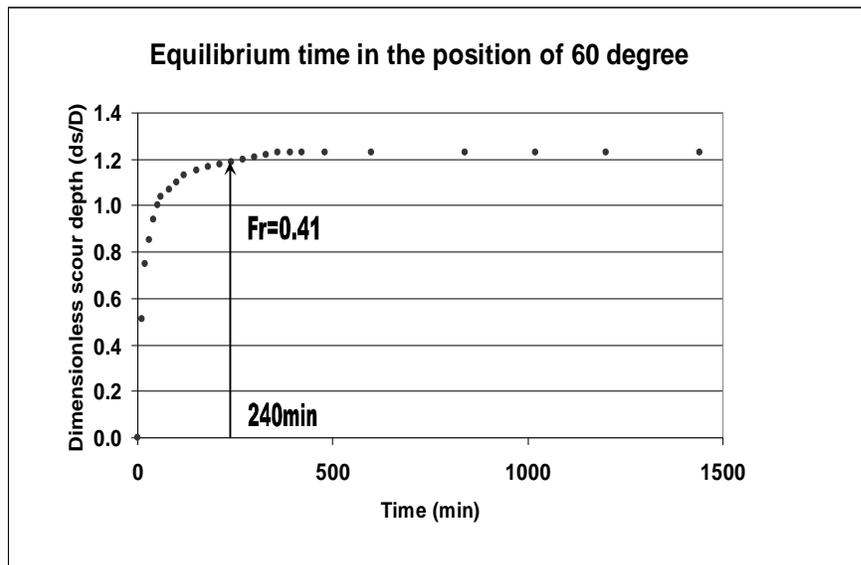
Figure 4. Equilibrium time in the position of 60 degree for a pier without collar
