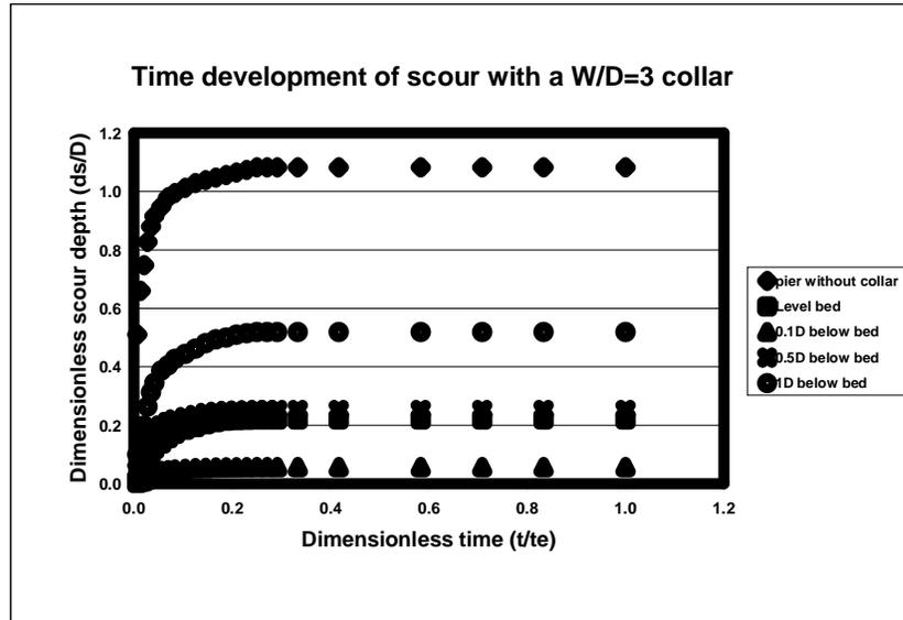
Figure 8. Time development of scour for different elevations
