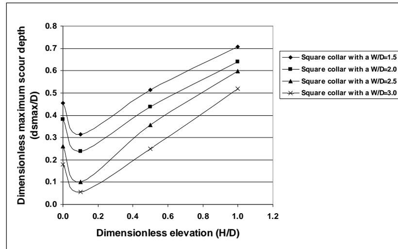
Figure 9. Maximum scour depth for different elevations
