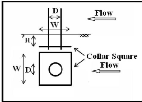
Figure 3. Circular pier fitted with a square collar
