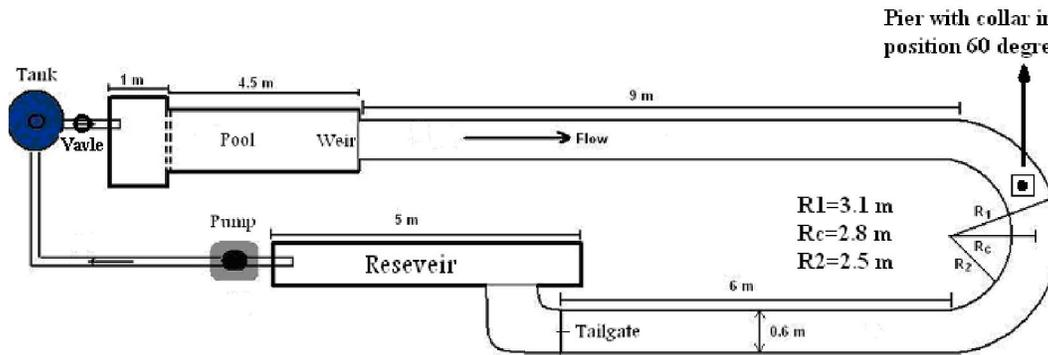
Figure 2. Illustration of the experimental setup (Plan)
