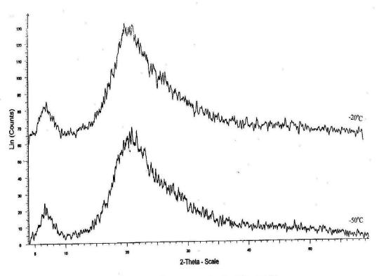
Fig.10 X-ray diffraction patterns of DPC at -20°C and -50°C.
