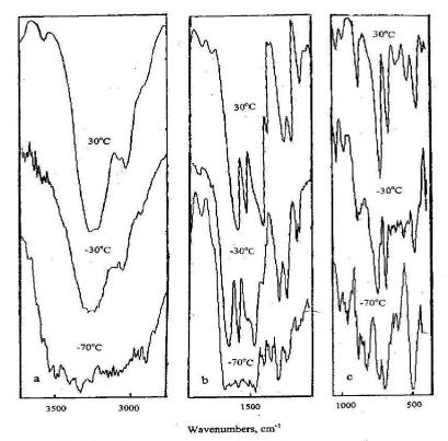
Fig.9 Variation of band shapes at a set of selected temperatures (-70°C, -30°C, 30°C) for DPC modes:a)Asymmetric stretching of N-H.
