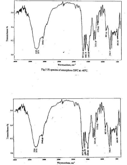
Fig.6 IR spectra of amorphous DPC at -30°C.
