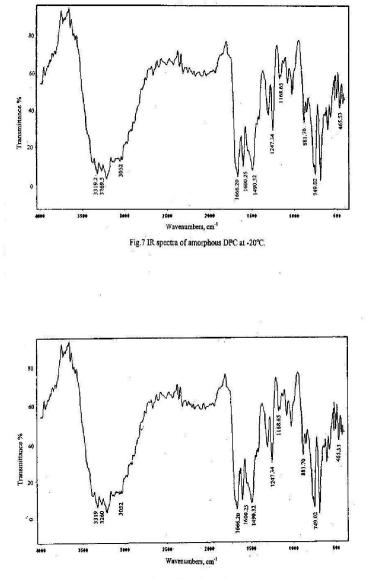
Fig.8 IR spectra of amorphous DPC at -10°C.
