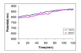
Fig-5 Potential vs. Time for sacrificial cathodic protection system to (Al - 4%Zn-0.4%Sn) in Al-Qasim solution
