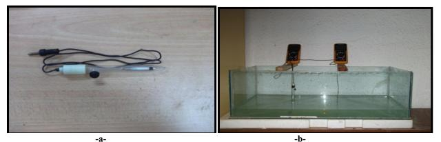
Fig-2 a: The Saturated Calomel Elec, b: Sacrificial cathodic protection system
