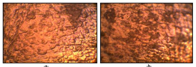
Fig-12 a: The microstructure of (Al – 4% Zn -0.4%Sn)alloy after immersion, 400X b:The microstructure of (Al – 4% Zn-0.5%Sn )alloy after immersion, 400X
