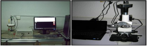
Fig-3 a: The Tafel tester to test electrochemical corrosion, b:Light Optical Microscopy (LOM).
