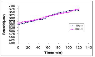
Fig-4 Potential vs. Time for sacrificial cathodic protection system to (Al – 4%Zn) in Al-Qasim solution
