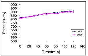
Fig-6 Potential vs. Time for sacrificial cathodic protection system to (Al – 4%Zn-0.5%Sn) in Al-Qasim solution
