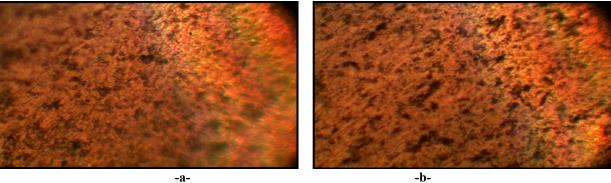
Fig-10 a: The microstructure of (Al – 4% Zn) alloy before immersion, 400X b: The microstructure of (Al – 4% Zn-0.4%Sn)alloy before immersion, 400X
