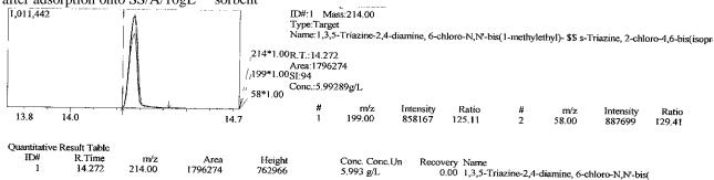
Figure 4: GC/MS chromatogram, quantitative measurement and spectral information of equilibrium phase atrazine after adsorption onto SS/A/15gL<sup>-1</sup> sorbent
