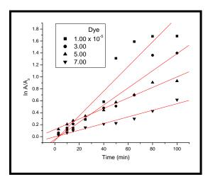
Fig. (2b) Kinetic of photodegradation of  $Fe^{2+}$  3.0 x  $10^{-5}$  at different initial concentrations of C.I. Mordant orange 1 in presence of 30.00 mM  $H_2O_2$  in photo-Fenton process and pH: 3.00.
