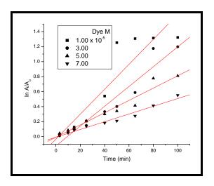
Fig. (2a) Kinetic of photodegradation of  $Fe^{2+}$  3.0 x  $10^{-5}$  at different initial concentrations of C.I. Mordant orange 1 in presence of 30.00 mM  $H_2O_2$  in Fenton process and pH: 3.00.
