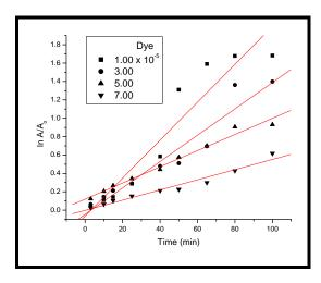
Fig. (2b) Kinetic of photodegradation of  $Fe^{2+}$  3.0 x  $10^{-5}$  at different initial concentrations of C.I. Mordant orange 1 in presence of 30.00 mM  $H_2O_2$  in photo-Fenton process and pH: 3.00.
