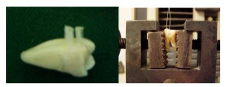
Figure 1: a, specimen with micro-cylenders bonded to buccal surface; b, <u>uSBS</u> compartments
