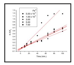
Fig. (4a): Kinetic of photodegradation of C.I. Mordant Orange 1 1.0 x  $10^{-5}$  M at different initial concentrations of Fe<sup>2+</sup> in presence of 30.00 mM  $H_2O_2$  Fenton process and pH: 3.00.
