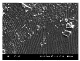
Figure 6. Low-magnification scanning electron photomicrography revealed small deposits on the curved-shape surface of silicon IOL
