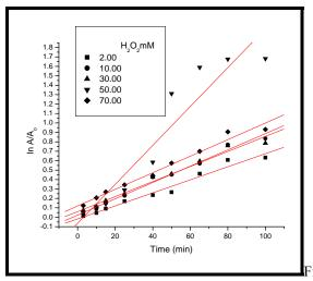
g. (3a): Kinetic of photodegradation of C.I. Mordant Orange 1 1.0 x  $10^{-5}$  M at different initial concentrations of  $H_2O_2$  in presence of  $Fe^{2^+}$ :  $3.0 \times 10^{-5}$  in Fenton process and pH: 3.00.
