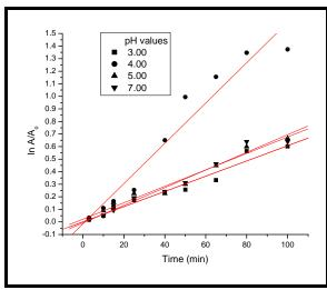
Fig. (5a): Kinetic of photodegradation of C.I. Mordant Orange 1 1.0 x  $10^{-5}$  M at different initial concentrations of pH values in presence of 30.00 mM  $H_2O_2$  Fenton process and  $Fe^{2+}$  3.0 x  $10^{-5}$  M
