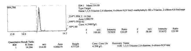
Figure 3: GC/MS chromatogram, quantitative measurement and spectral information of equilibrium phase atrazine after adsorption onto  $SS/A/10gL^{-1}$  sorbent
