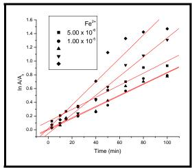
Fig. (4b): Kinetic of photodegradation of C.I. Mordant Orange 1 1.0 x  $10^{-5}$  M at different initial concentrations of Fe<sup>2+</sup> in presence of 30.00 mM  $H_2O_2$  photo-Fenton process and pH: 3.00.
