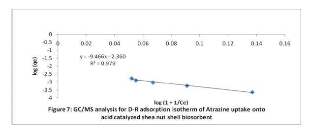
The R-D Theoretical saturation capacity,  $q_D$  and the Langmuir maximum adsorption capacity,  $q_m$  were both estimated as  $q_D = 4.37 \times 10^{-3} \, \text{mgg}^{-1}$  and  $q_m = 0.772 \times 10^{-3} \, \text{mgg}^{-1}$ . No known and proven reference could make us conclude that the theoretical saturation capacity,  $q_D$  is always higher than the maximum adsorption capacity as the case was made evidence in this research.
