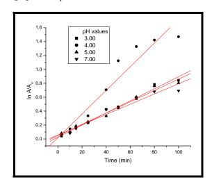
Fig. (5b): Kinetic of photodegradation of C.I. Mordant Orange 1 1.0 x  $10^{-5}$  M at different initial concentrations of pH values in presence of 30.00 mM  $H_2O_2$  Photo-Fenton process and  $Fe^{2+}$  3.0 x  $10^{-5}$  M
