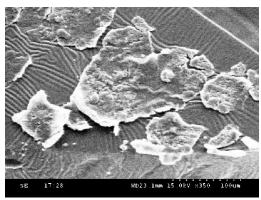
Figure 7. The deposits forming amorphous crustlike layer on the posterior optic surface of the lens under high-magnification scanning electron photography.
