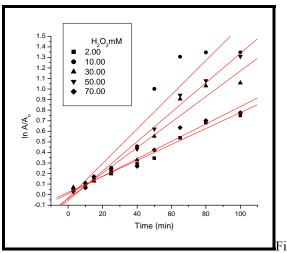
g. (3b): Kinetic of photodegradation of C.I. Mordant Orange 1 1.0 x  $10^{-5}$  M at different initial concentrations of  $H_2O_2$  in presence of  $Fe^{2^+}$ :  $3.0 \times 10^{-5}$  in Photo-Fenton process and pH: 3.00.
