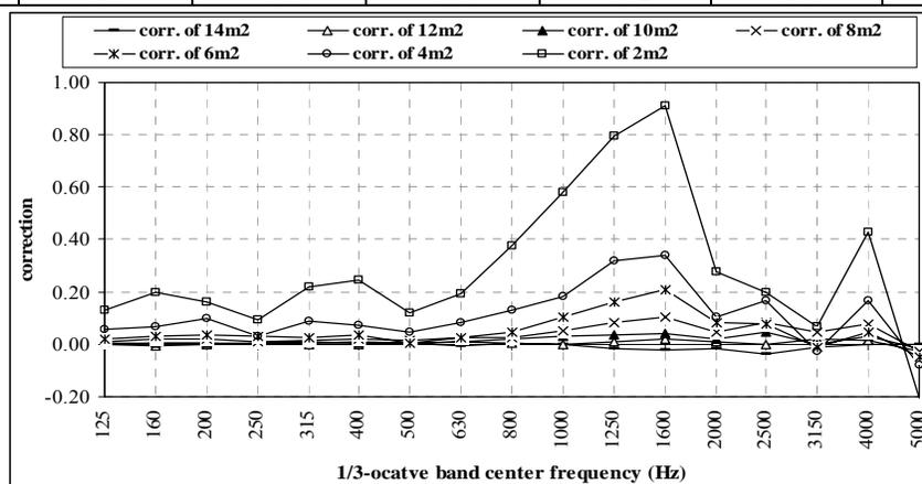
**Fig.2d: absorption correction surface area for polyisoprene material****4- Conclusion**
