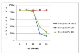
Fig. 3 Throughput Vs No. of Nodes for Packet sizes 1024 bytes
