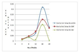
Fig. 6 End to End Delay Vs. No. of Nodes for Packet sizes 1024 bytes
