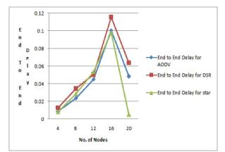
Fig. 5 End to End Delay Vs No. of Nodes for Packet sizes 512 bytes.
