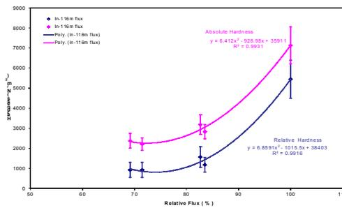
**Fig.(5): Represent the relation between the flux and the hardness of stainless steel foils.**
