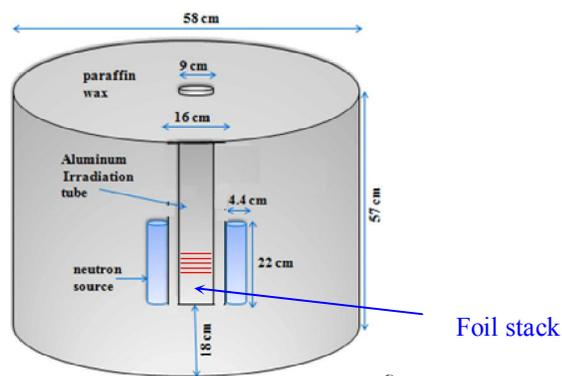
Fig. (1): The layout of Am-Be neutron irradiation facility used in this work<sup>(4-6)</sup>.
