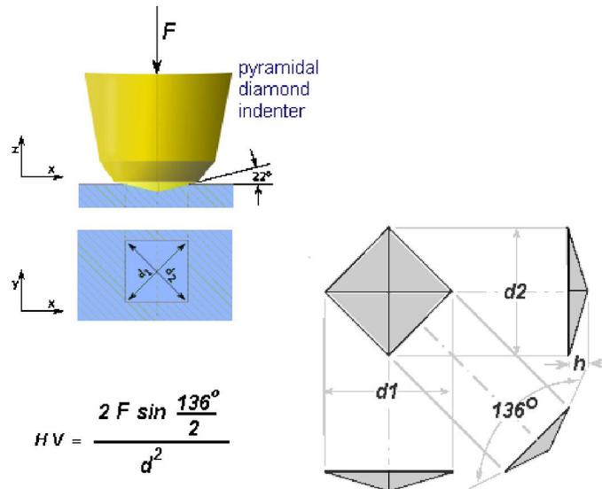
Fig. (2): Vickers hardness test scheme.
