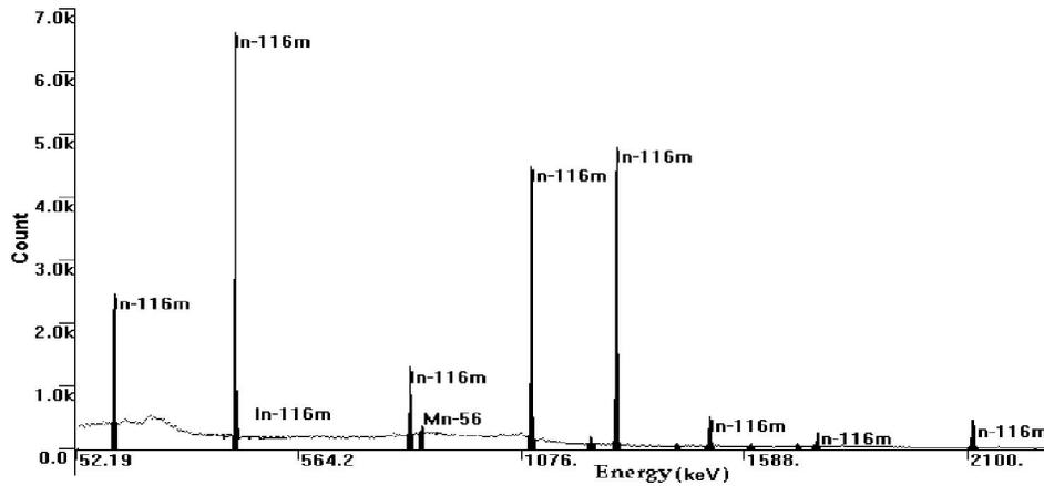
**Fig.(3):** Gamma spectrum of activated indium foil measured using 70% HPGe.
