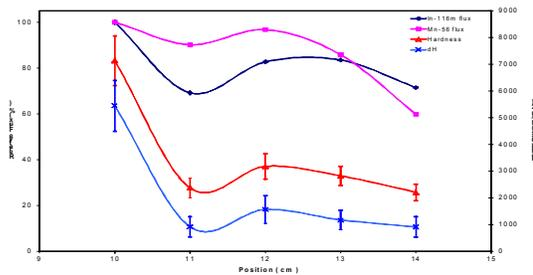
**Fig.(4):** Represent thermal neutron flux distribution in the irradiation chamber.
