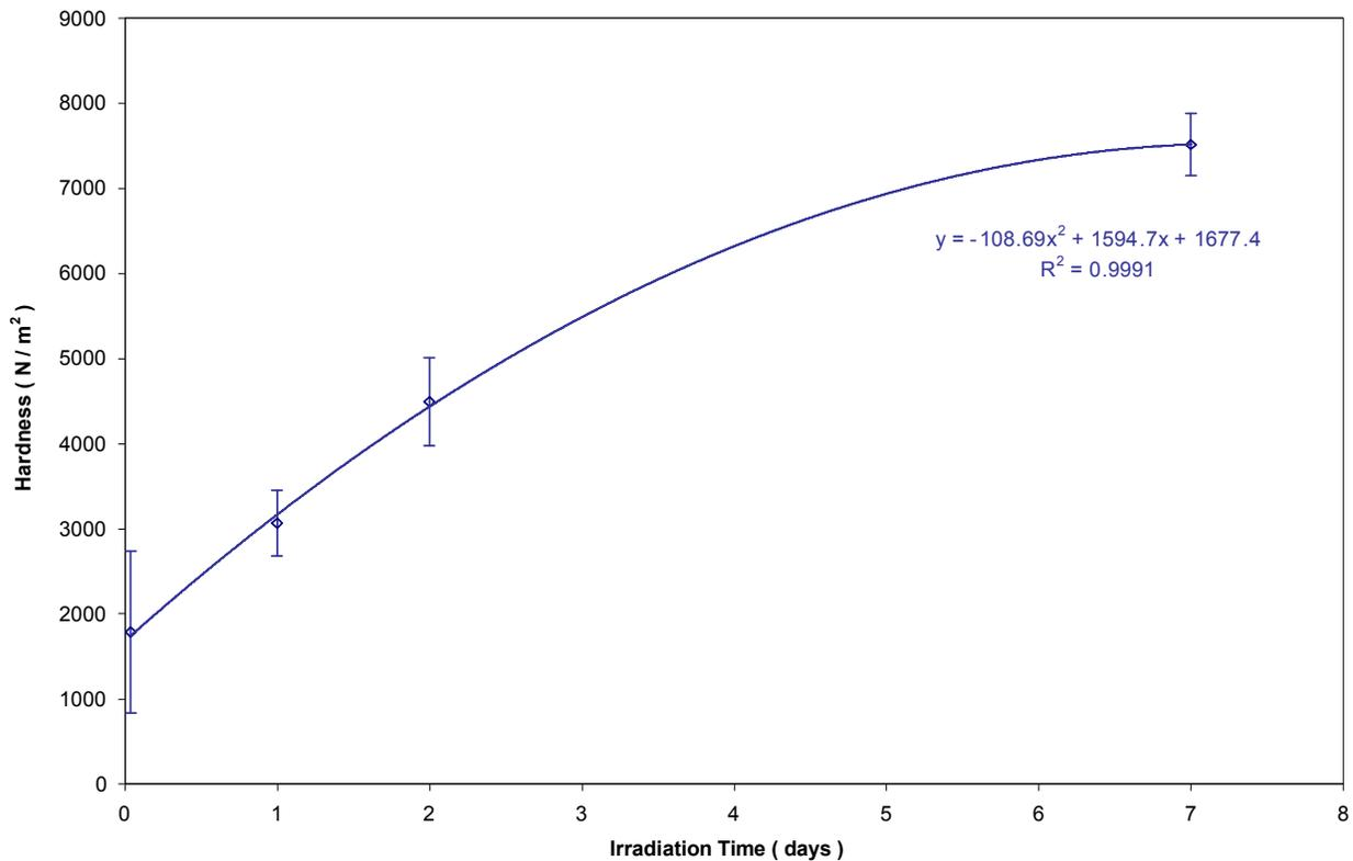
**Fig.(8): Represent neutron Flux dependence of hardness increment**
