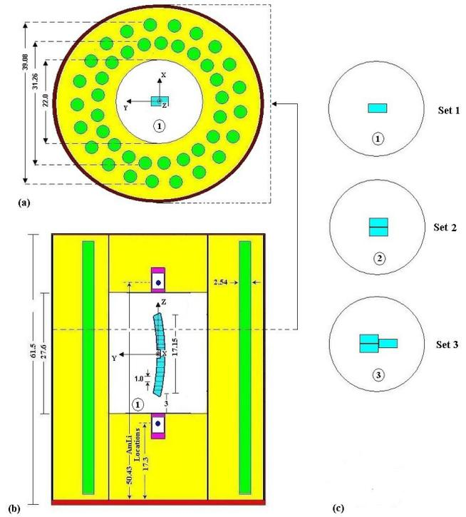
Figure 2. Geometrical model of the AWCC used for Monte Carlo calculations with different setup configurations of DU metal samples inside the cavity. (a) Cross sectional view, (b) longitudinal view and (c) different setup configuration for different sets.
