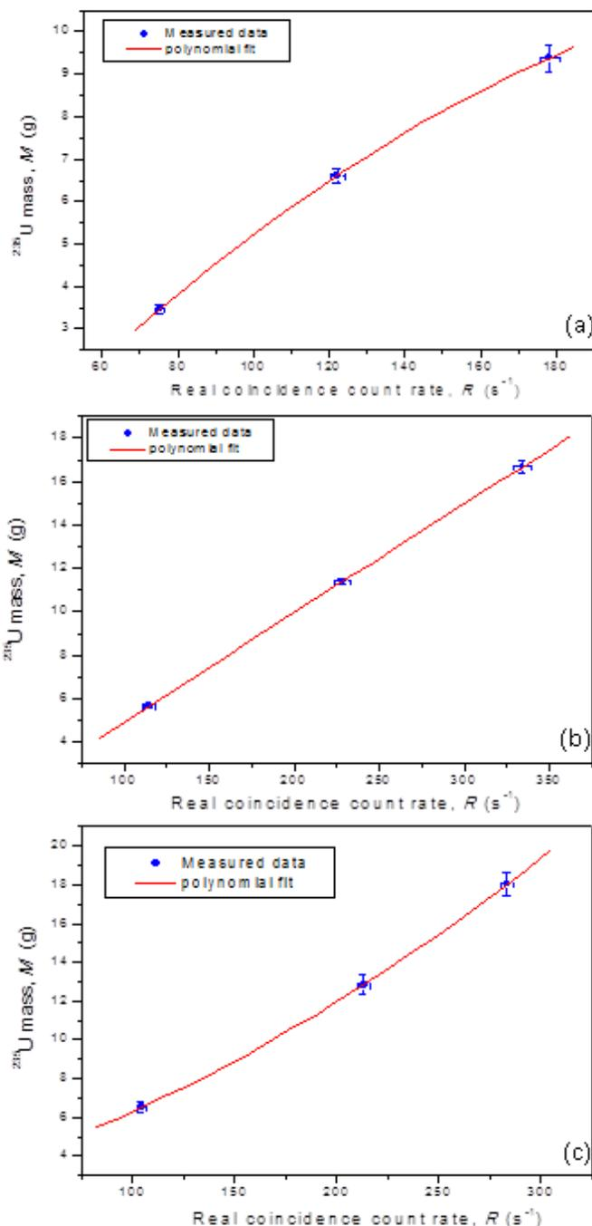
Figure 7. The variation of the real coincidence count rate with  $^{235}\text{U}$  mass. Solid line represents the second order polynomial fit of the estimated data (a)  $(\text{NH}_4)_2\text{U}_2\text{O}_7$  matrix, (b)  $\text{UF}_4$  matrix and (c) DU metal.
