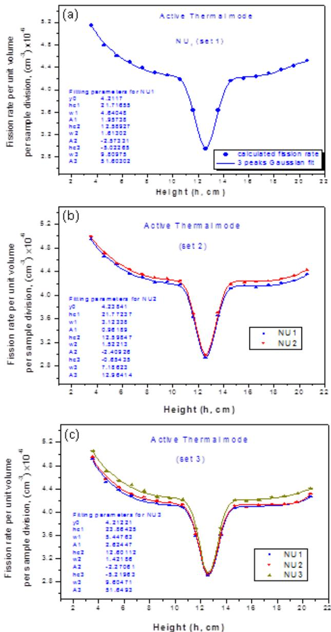
Figure 5 (a-c). The calculated fission rates per unit volume per NM sample division for each sample and setup configuration for UF<sub>4</sub> matrix.
