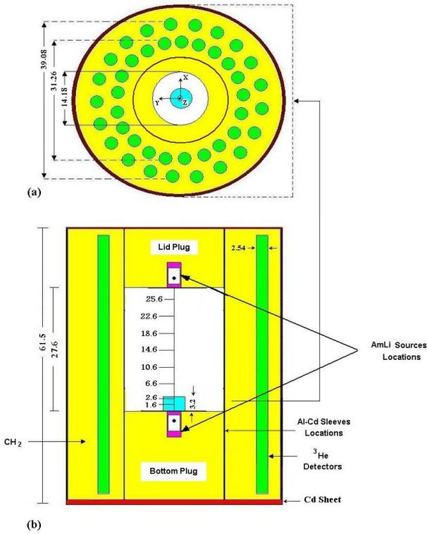
Figure 1. Experimental setup configuration for 1.068 kg NU metal sample measured inside the detector cavity to obtain the efficiency in active thermal mode by removing the insert Al-Cd sleeves (a) Cross sectional view, (b) longitudinal view.
