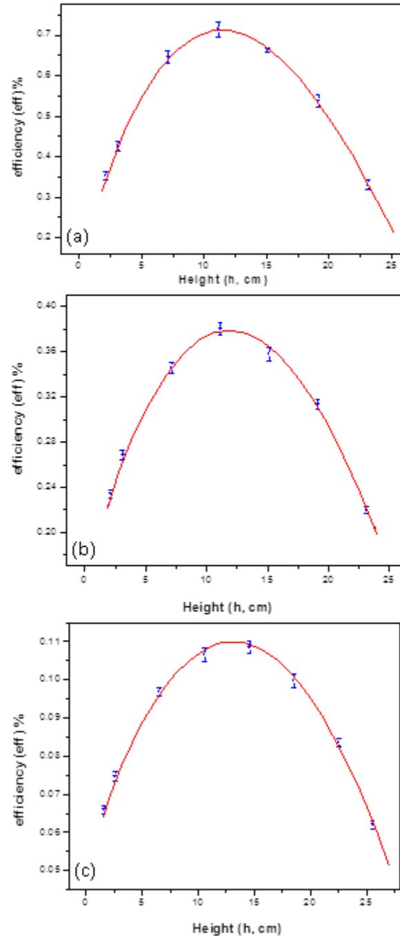
Figure 3. The variation of the measured coincidence efficiency of the detector using the characterized sample with location inside the detector cavity for (a)  $(\text{NH}_4)_2\text{U}_2\text{O}_7$  matrix (b)  $\text{UF}_4$  matrix (c) DU metal.
