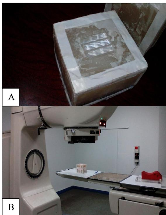
Figure 1. The cubic phantom (A) the two parts of wax phantom, (B) the phantom at the top of cobalt60 treatment machine.
