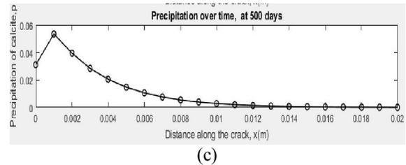
Figure 8: Precipitation of calcite (a) 20 days, (b) 200 days, (c) 500 days
