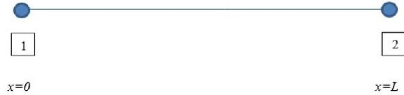
Figure 4. Linear bar element
