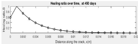
Figure 11: Healing ratio,  $S=100\%$  at  $c_0=750 \text{ mole/m}^3$  and time 450 days
