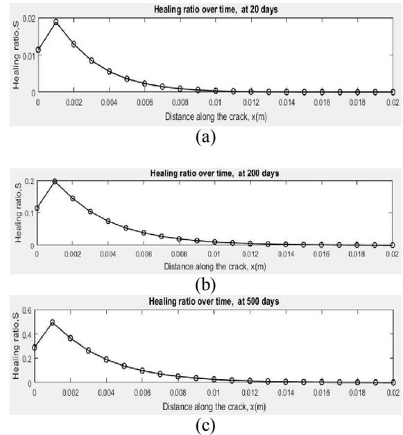
Figure 9: Healing ratio at (a) 20 days = 17%, (b) 200 days = 20%, (c) 500 days = 50%
