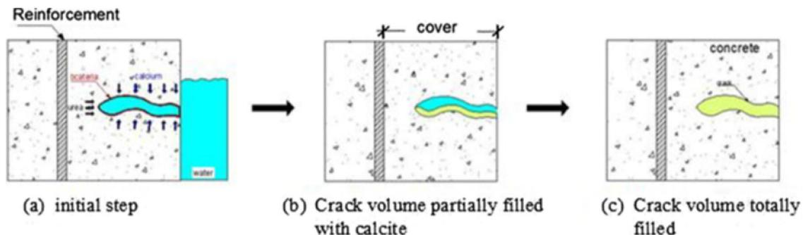
Figure 1. The development of a crack repairing over various stages
