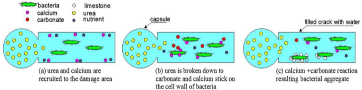
Figure 2. Schematic diagram of evolving microbial calcium carbonate (CaCO<sub>3</sub>), Algaifi (2018)
