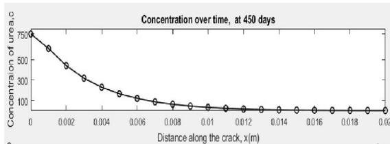
Figure 10: Concentration of urea,  $c_0=750 \text{ mole/m}^3$
