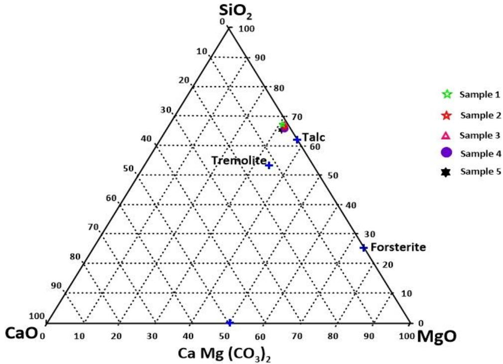
Figure 4: Ternary diagram of CaO – SiO<sub>2</sub> – MgO (Modified after Tahir *et al.*, 2018).
