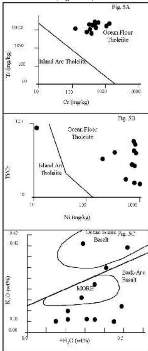
Fig. 5 Plots of mafic rocks of Winder area showing tectonic affiliation, A) Ti vs. Cr (after Pearce, 1975); B) Ni vs. Ti/Cr ratio (after Beccaluva et al., 1979); C) H<sub>2</sub>O vs. K<sub>2</sub>O (tectonic boundaries after Rollinson, 1993).
