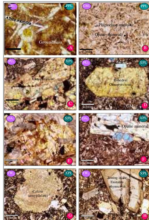
Fig. 2 Photomicrographs of mafic igneous rocks of the Winder area. Sample numbers are marked on top left and status of nicols on top right.
