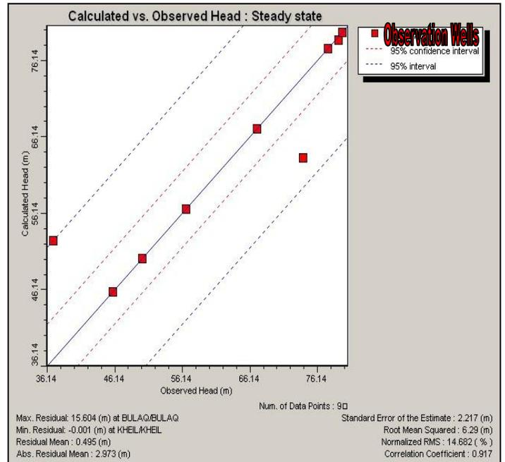
Figure 8: Results of the Steady State Calibration
