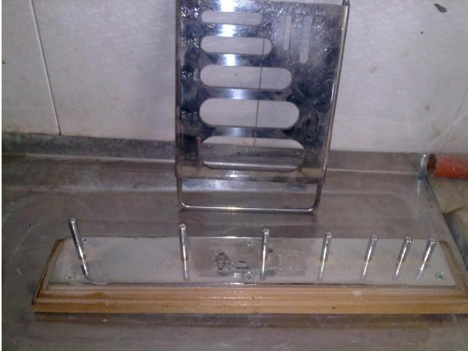
Figure 3.4: prolongation and browsing devices to test needle and flake materials
