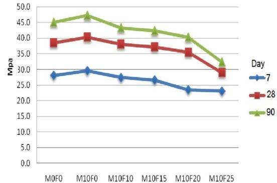
Fig. 5.1: compressive strength of fly ash samples with increasing substitution of different ages
