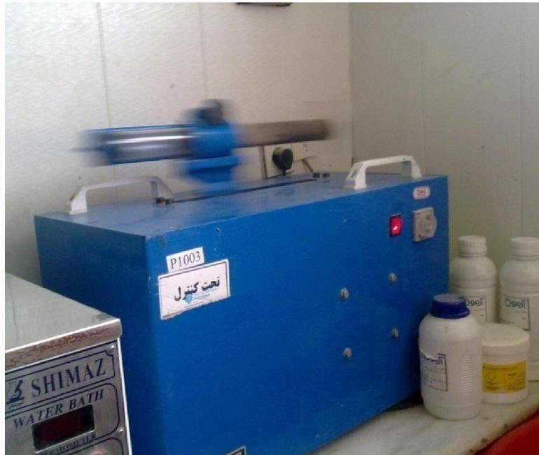
Figure2.4 - shaker device for determination of sandy materials
