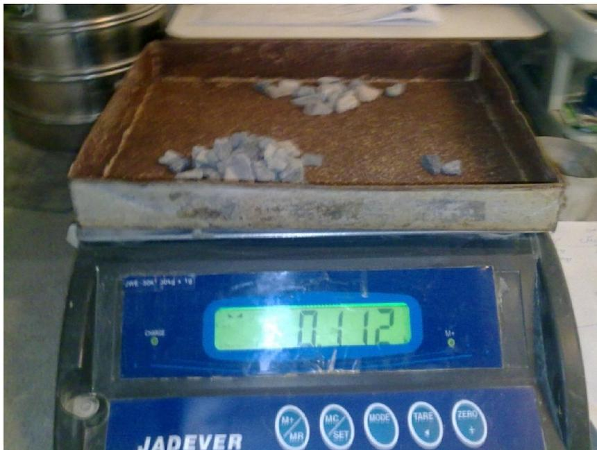
Figure 4.4: weight of the sample to determine the amount of material flake and needle
