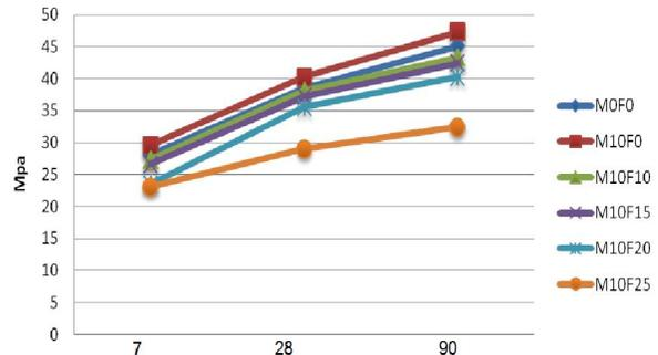
Fig 5.2: compressive strength of samples over time
