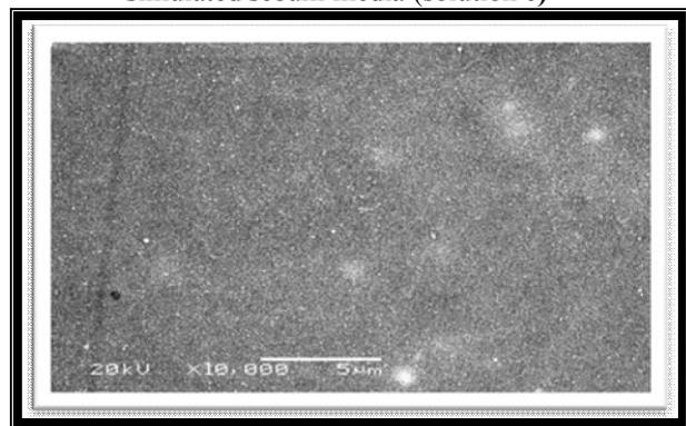
**Figure 5.** SEM of control group (distilled water) smooth surface with some scattered particles at (10,000 X) magnification
