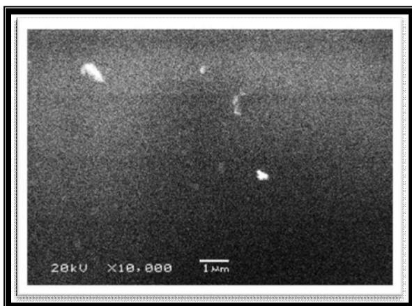
**Figure 8.** SEM of group IV (simulated sebum) showed smooth grazed surface with some scattered particles at (10,000 X) magnification
