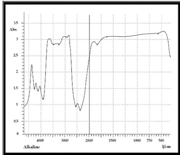
**Figure 3.** FTIR analysis for test Group III stored in a simulated alkaline media (solution b)
