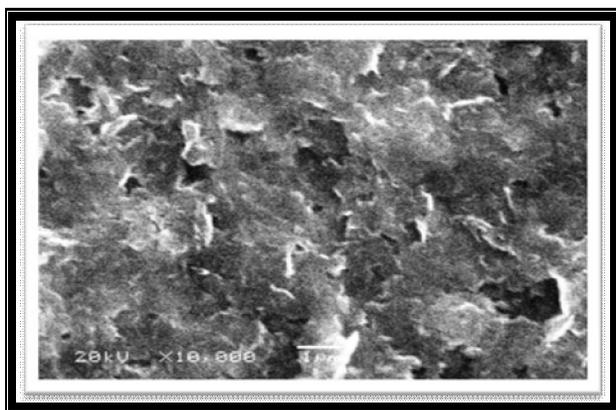
**Figure 7.** SEM of group III (simulated alkaline) showed irregular vacuolated surface at (10,000 X) magnification
