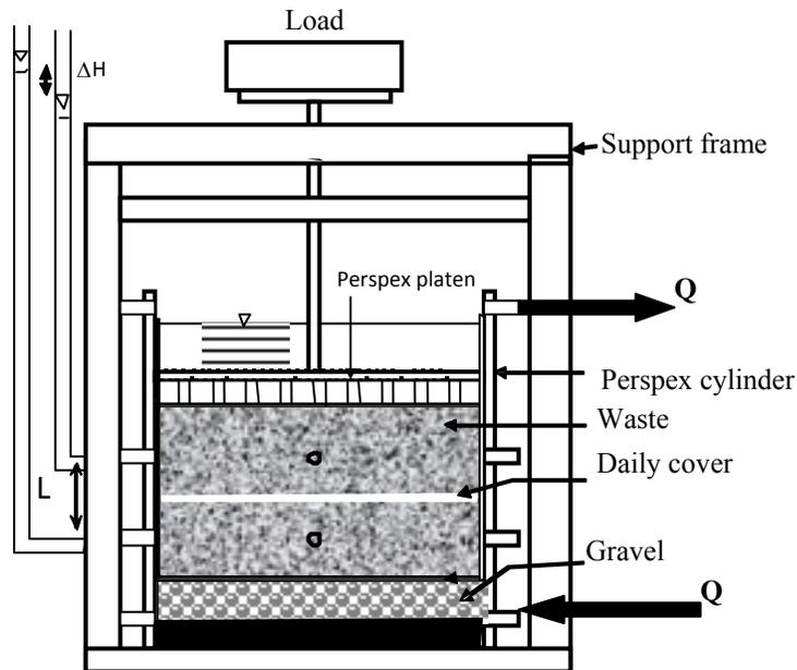
Figure 1: The small compression cell unit used for the hydro-physical tests on municipal solid refuse (Oni, 2000)
