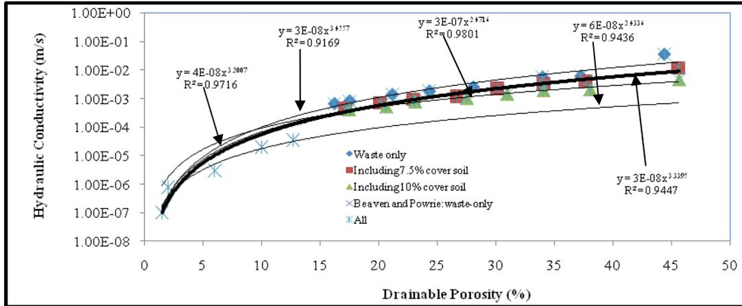
Figure 5: The plots and characteristic trends of saturated hydraulic conductivity versus porosity for the municipal solid refuse
