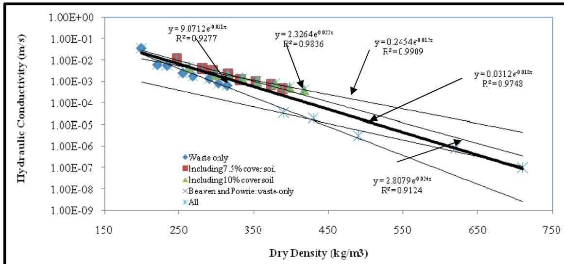
Figure 3: The plots and characteristic trends of saturated hydraulic conductivity versus dry density for the municipal solid refuse
