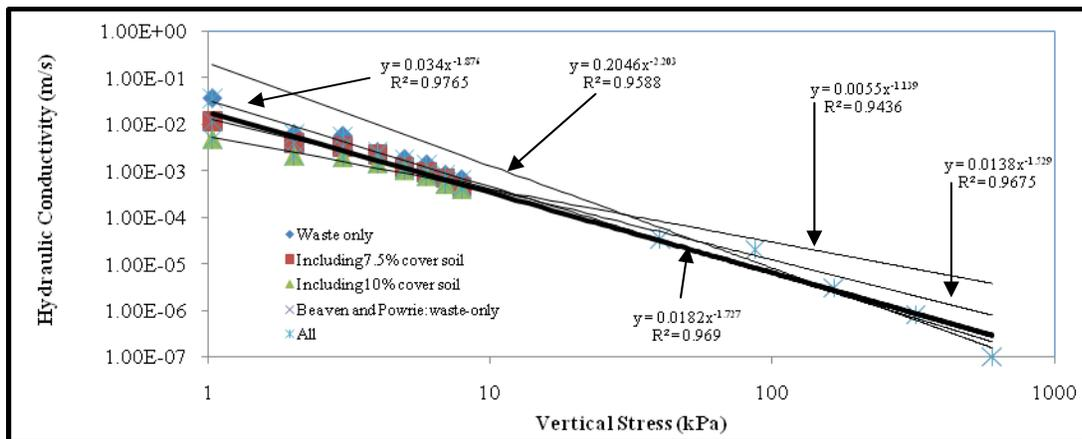
Figure 6: The plots and characteristic trends of saturated hydraulic conductivity versus vertical stress for the municipal solid refuse
