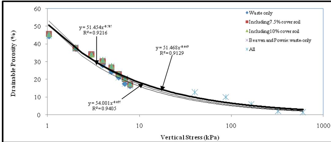
Figure 8: The plots and characteristic trends of drainable porosity versus vertical stress for the municipal solid refuse
