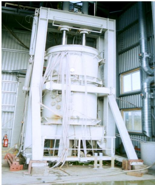
Figure 2: The large-scale Pisea compression cell unit used for the hydro-physical tests on municipal solid refuse (Beaven, 2000; Hudson, 2010)
