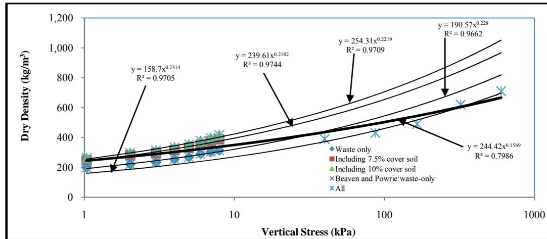
Figure 7: The plots and characteristic trends of vertical stress versus dry density for the municipal solid refuse
