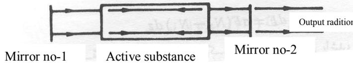
Fig2- the laser resonator
