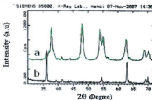
**Figure 2.** XRD pattern of surfaces of TiO<sub>2</sub> thin films annealed at 450 °C (a) and 750 °C (b).
