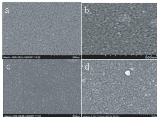
**Figure 1.** FE-SEM images of annealed TiO<sub>2</sub> thin film surfaces at (a) 300 °C, (b) 400 °C, (c) 450 °C and (d) 750 °C.
