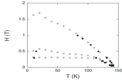
Fig. 2 Fields at which magnetization jumps were observed at different temperatures in field sweeps (circles) and temperature sweeps (squares). Diamonds represent jumps in temperature sweeps that yielded magnetization jumps already during the field sweep at 10 K.
