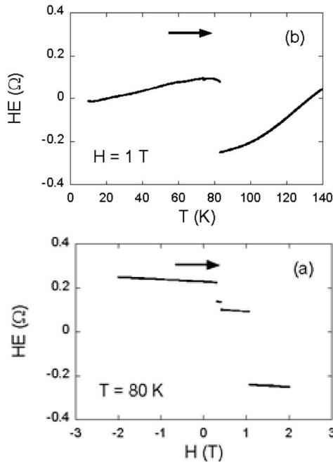
Fig. 1 (a) Hall effect vs H at 80 K after cooling in a field  $-2$  T from above  $T_C$ . (b) Hall effect vs temperature after cooling in a field of  $-2$  T from above  $T_C$  down to 10 K and setting the field to 1 T at that temperature.
