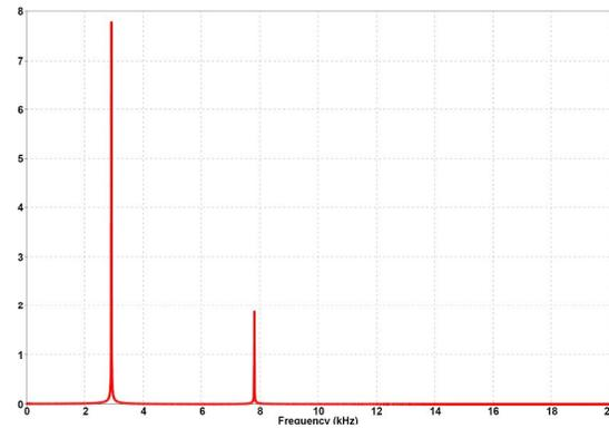
Figure 11. Frequency response for C11=12nF and C1n=16nF, Case: without fault
