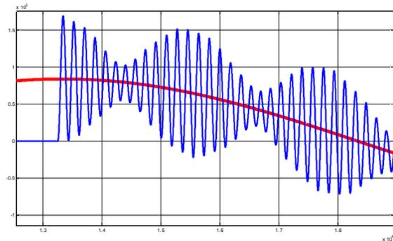
Figure 1. Power frequency (dot) versus the TRV oscillations frequency (solid)
