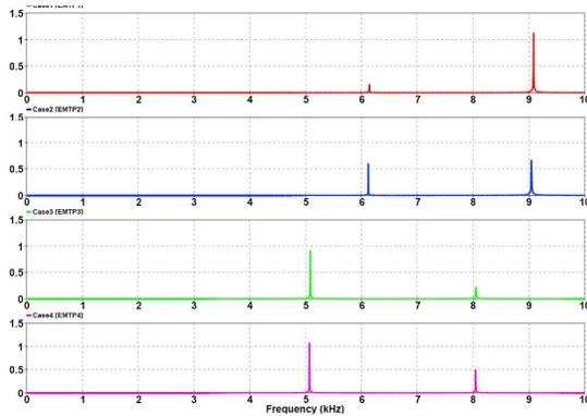
Figure 10. Frequency response by increasing the capacitance of C1n
