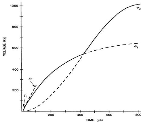
Figure 3. TRV envelope curve
