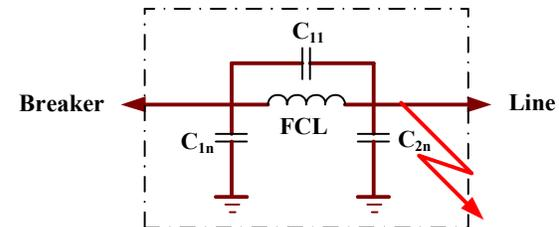
Figure 5. Fault current Limiter and TRV requirements
