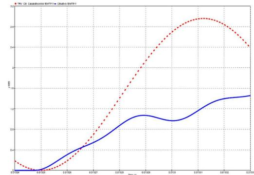
Figure 6. TRV (solid) and Capability Curve (dotted),  $C_{11}=9\text{nF}$
