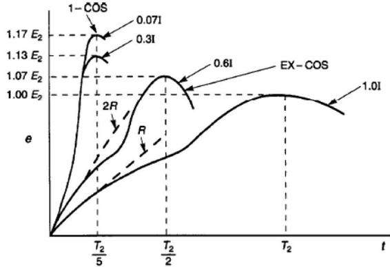
Figure 2. CB curves for 121kV voltage levels and above
