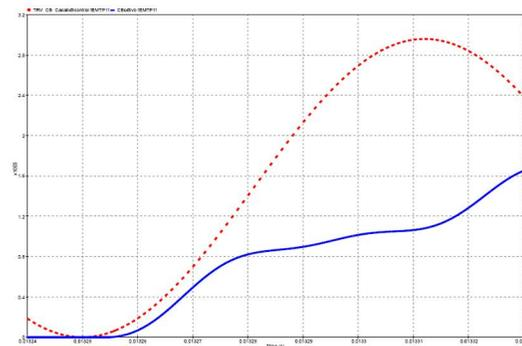
Figure 7. TRV (solid) and Capability Curve (dotted),  $C_{11}=12\text{nF}$
