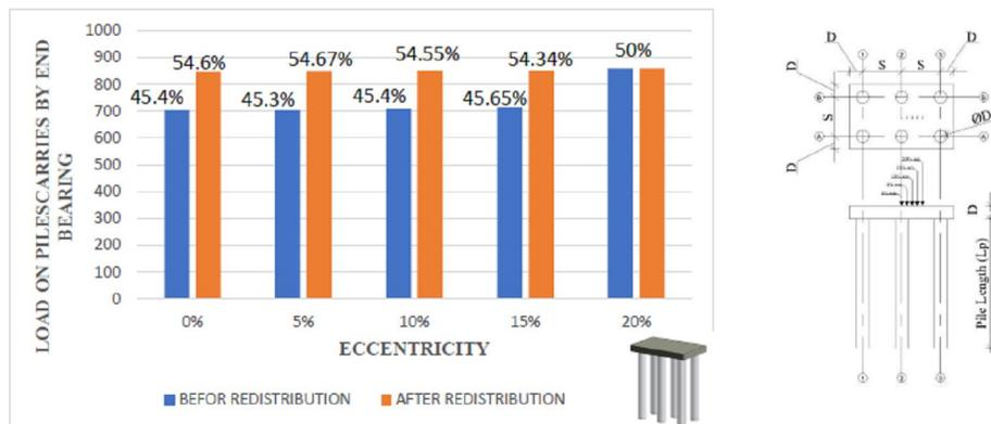
FIG. (58) COMPARISON BETWEEN LOAD ON PILES CARRIED BY END BEARING BEFOR AND AFTER REDISTRIBUTION AT DIFFERENT ECCENTRICITY IN X-DIRECTION AT (Lp=38D, D=0.6 M AND Sp=3D)
