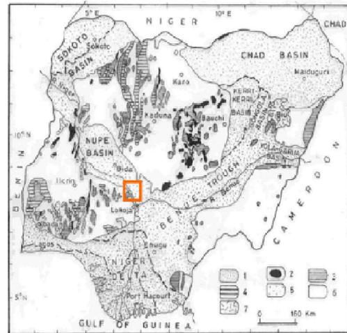
**Fig. 1.1 Geological map of Nigeria, 1 = Cretaceous-Recent sediments; 2=Younger Granites; 3 = Older Granites; 4 = Undifferentiated Metasediments; 5 = quartzite and quartzite schist; 6 = Undifferentiated basement complex and 7 = Tertiary volcanics (From Geological map of Nigeria 1994: compiled by the Geological Survey of Nigeria). Inset is the study area: the Koton Karifi Area of the Nupe Basin, Nigeria**
