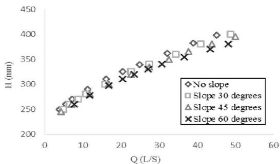
Figure 11. Comparison relationship between discharge and upstream head at 4 upstream slopes in model 2
