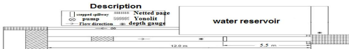
Figure 1. Water circulation system in the experimental flume
