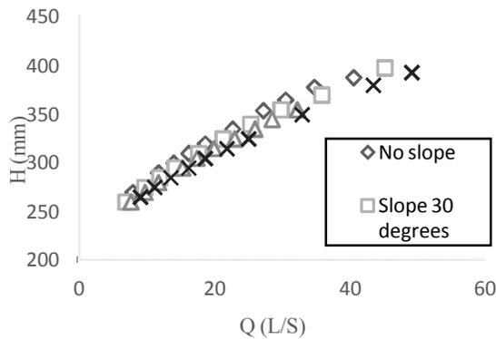
Figure 6. Comparison relationship between discharge and upstream head at 4 upstream slopes in model 1
