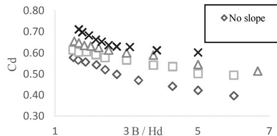
Figure 13. Comparison the relationship between  $C_d$  and  $\frac{B}{H_d}$  at 4 upstream slopes in model 2
