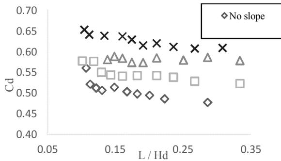
Figure 9. Comparison the relationship between  $C_d$  and  $\frac{L}{H_d}$  at 4 upstream slopes in model 1
