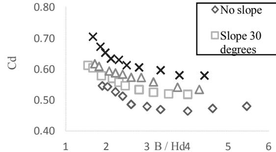
Figure 18. Comparison the relationship between  $C_d$  and  $\frac{B}{H_d}$  at 4 upstream slopes in model 3
