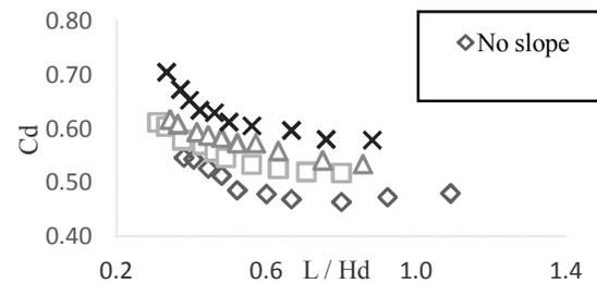
Figure 19. Comparison the relationship between  $C_d$  and  $\frac{L}{H_d}$  at 4 upstream slopes in model 3
