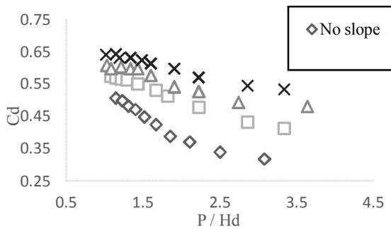
Figure 22. Comparison the relationship between  $C_d$  and  $\frac{P}{H_d}$  at 4 upstream slopes in model 4
