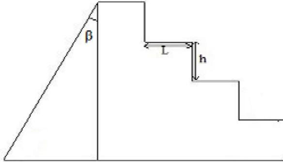
Figure 2. Schematic view a stepped spillway with slope upstream
