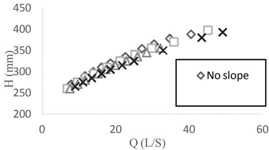
Figure 21. Comparison relationship between discharge and upstream head at 4 upstream slopes in model 4
