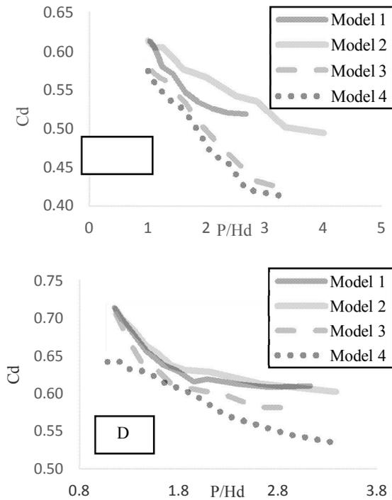
Figure 25. Comparison the relationship between Cd and  $\frac{P}{H_d}$  at 4 stepped spillway models in upstream slopes- A. No slope, B. Slope (30 degree), C. Slope (45 degree), D. Slope (60 degree)
