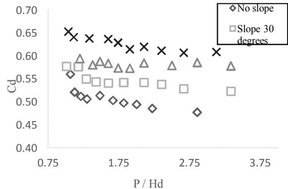
Figure 7. Comparison the relationship between Cd and  $\frac{P}{H_d}$  at 4 upstream slopes in model 1
