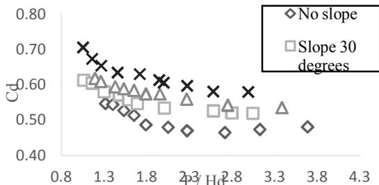
Figure 17. Comparison the relationship between  $C_d$  and  $\frac{P}{H_d}$  at 4 upstream slopes in model 3
