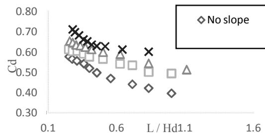
Figure 14. Comparison the relationship between  $C_d$  and  $\frac{L}{H_d}$  at 4 upstream slopes in model 2
