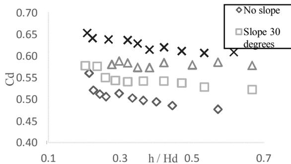
Figure 10. Comparison the relationship between  $C_d$  and  $\frac{h}{H_d}$  at 4 upstream slopes in model 1
