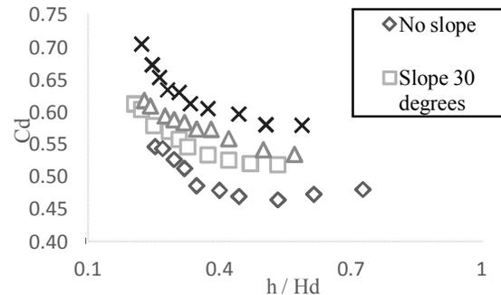
Figure 20. Comparison the relationship between  $C_d$  and  $\frac{h}{H_d}$  at 4 upstream slopes in model 3
