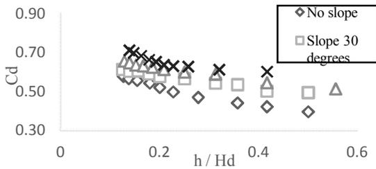
Figure 15. Comparison the relationship between  $C_d$  and  $\frac{h}{H_d}$  at 4 upstream slopes in model 2
