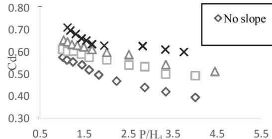
Figure 12. Comparison the relationship between  $C_d$  and  $\frac{P}{H_d}$  at 4 upstream slopes in model 2
