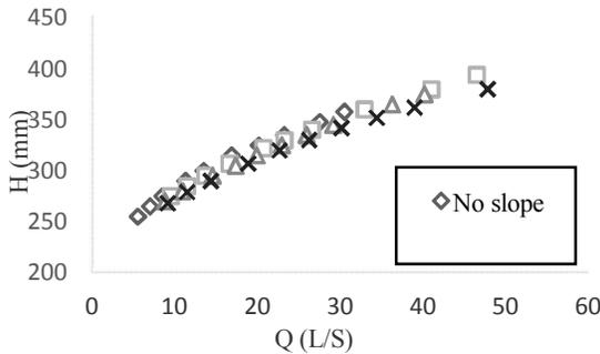
Figure 16. Comparison relationship between discharge and upstream head at 4 upstream slopes in model 3
