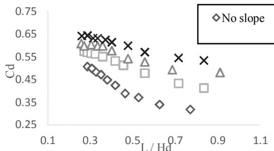
Figure 23. Comparison the relationship between  $C_d$  and  $\frac{L}{H_d}$  at 4 upstream slopes in model 4
