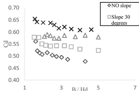
Figure 8. Comparison the relationship between Cd and  $\frac{B}{H_d}$  at 4 upstream slopes in model 1
