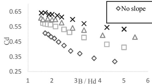
Figure 24. Comparison the relationship between  $C_d$  and  $\frac{B}{H_d}$  at 4 upstream slopes in model 4
