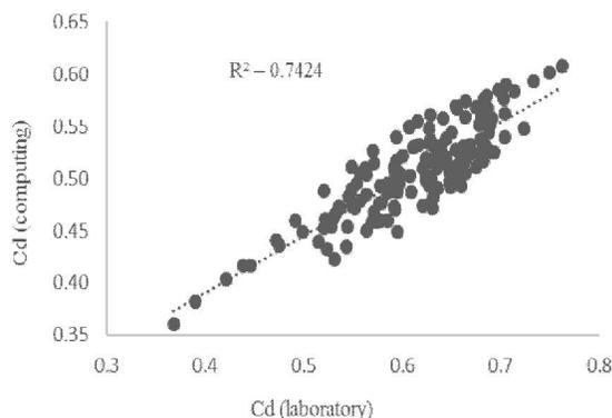
Figure 26. Comparison results of computing and laboratory of discharge coefficient in the Stepped spillway for measured data
