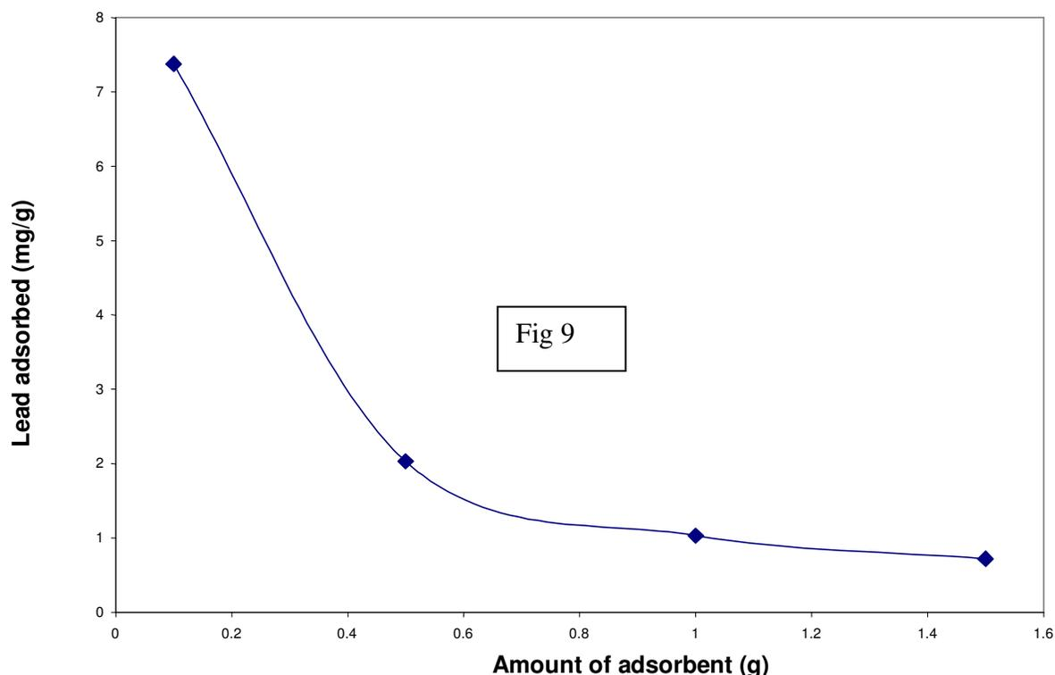
Figure 9. Effect of lead adsorbed on adsorbent dose at 25<sup>o</sup>C.
