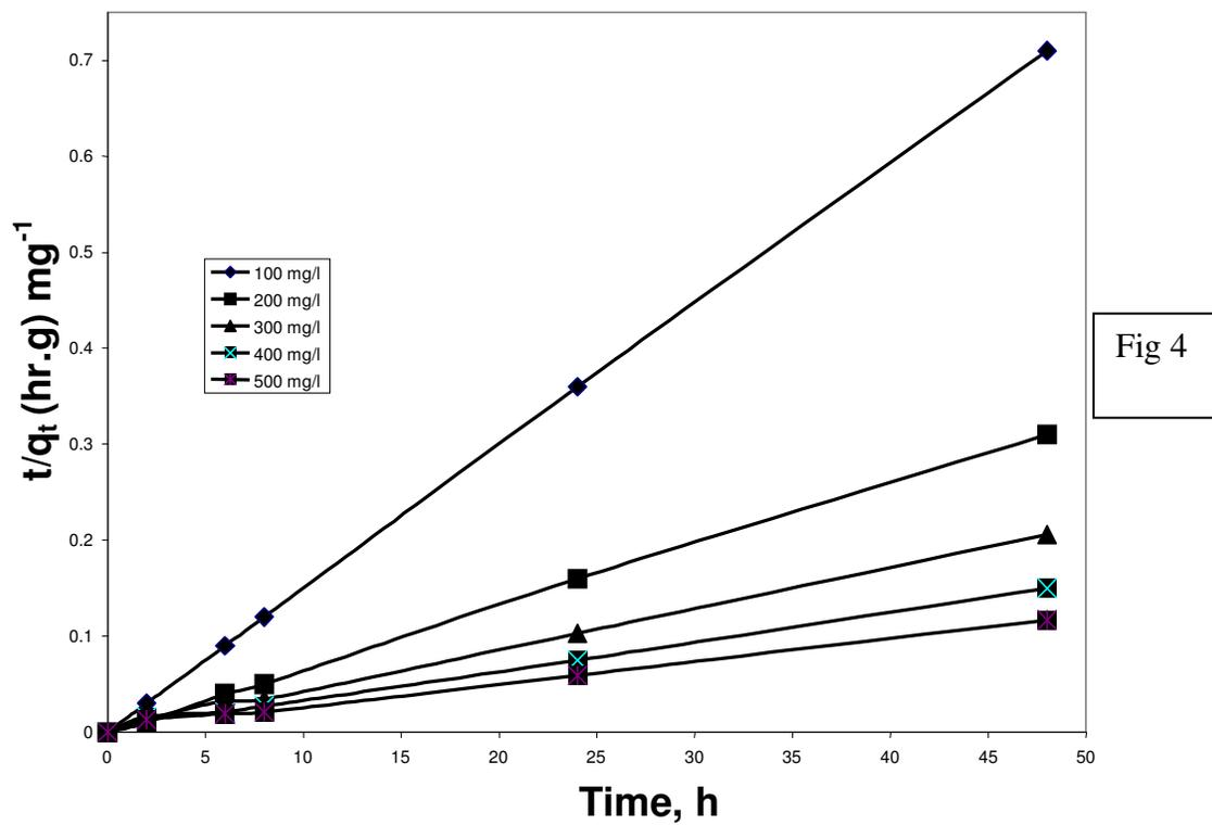
Figure 4. Pseudo-second order kinetics for adsorption of lead by activated carbon produced from treated oil palm fibre at 25°C.
