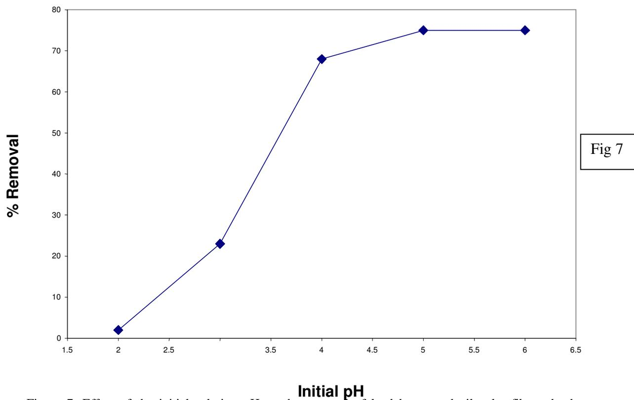
Figure 7. Effect of the initial solution pH on the removal of lead by treated oil palm fibre adsorbent (temperature 25<sup>0</sup>C; adsorbent concentration 5 g/L; initial dye concentration 100 mg/L).
