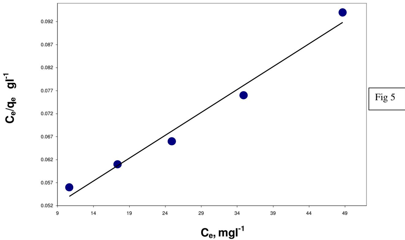
Figure5. Langmuir adsorption isotherm of lead on activated carbon produced from treated oil palm fibre at 25°C.
